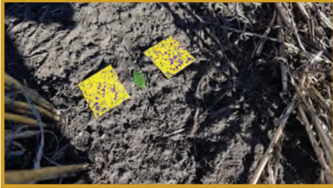
Water sensitive paper can be used to show whether a target has been detected (and therefore sprayed).
