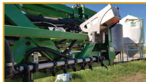
Older generation WEEDit sensors were placed at 1 m intervals and had five channels, each covering a 20 cm band. There were 180 nozzles on a 36 m (120 ft.) boom.
