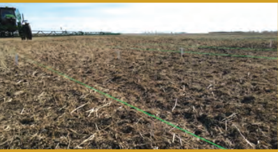
Monofilament strings can be used to collect spray over long distances.
