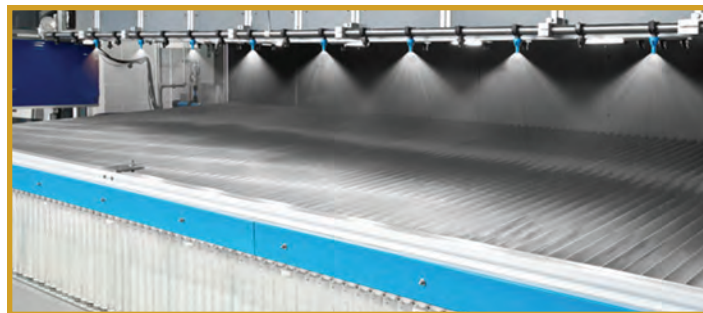
A spray patternator determines the uniformity of a stationary boom's spray distribution (Photo: TeeJet)
