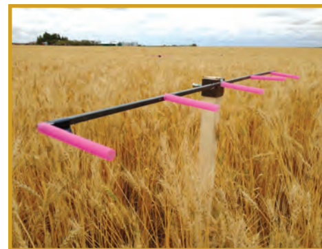
Plastic straws can act as collectors of sprays under field conditions.
