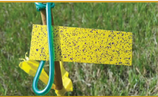
Water-Sensitive paper provides a quick visual indication of the deposit, not just amount but also qualitative aspects such as droplet size and distribution.
